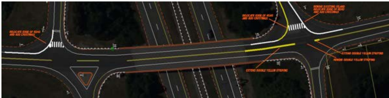
Figure 30. Sketch of potential SR 1 and SR 36 interchange improvements to accommodate bicyclists on the north/westbound side of Cedar Beach Road
